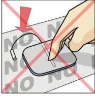
Do not place Electrodes on the "NO" side of the Release Liner.
