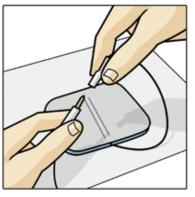
While disconnecting or inserting pin, hold the pin connector
