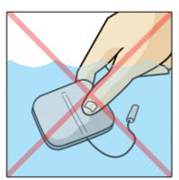
Do not submerge Electrodes in water.
