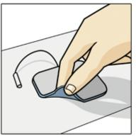
Remove Electrodes by lifting the edge.
