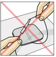
Do not pull the leadwire to remove the pin.
